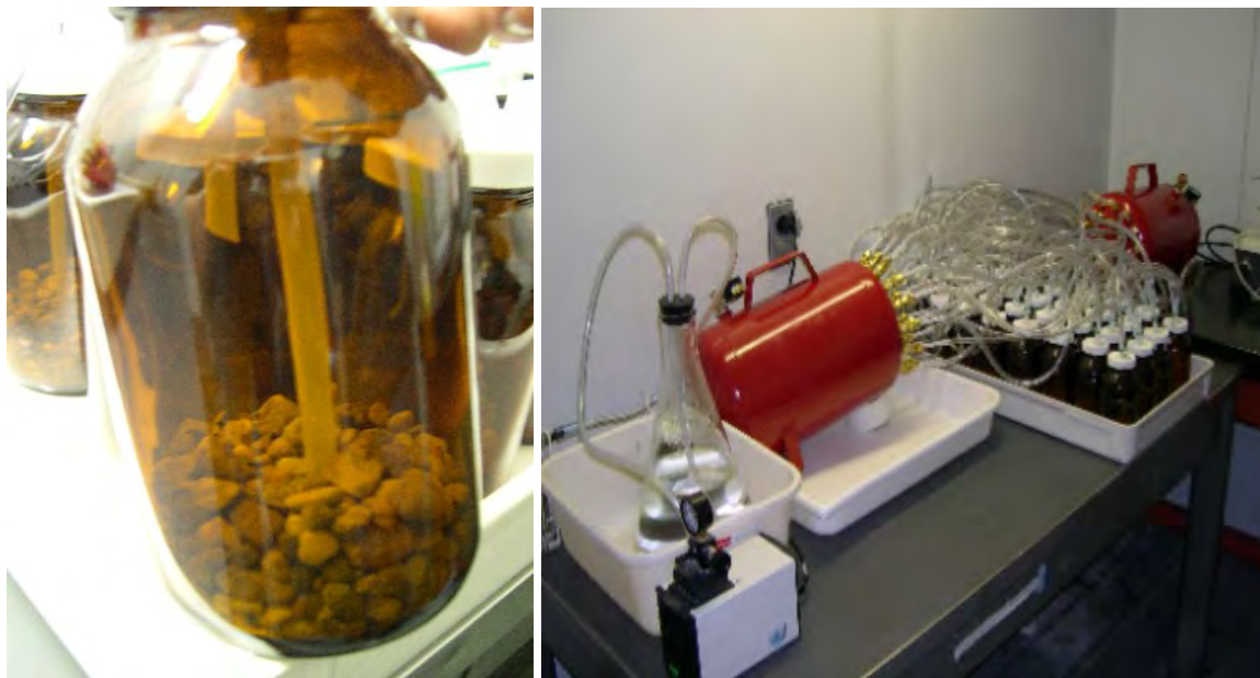
Figure 2.1 Photos of the temperature controlled reactor. The left photo shows a close up of the 0.5L reactors. The photo shows the entire apparatus including the air humidifying operation, the air distribution manifolds and the 36 reactors.
