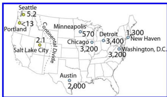
Figure 2. PAHs in dust swept from sealcoated parking lots show a striking geographic difference. PAH concentrations in dust from parking lots in central and eastern U.S. cities, where coal-tar-based sealcoat is commonly used, are about 1000 times higher than in the western U.S., where asphalt-based sealcoat is more commonly used. Concentrations are the sum of 12 PAHs ( \Sigma\text{PAH}_{12} ), in mg/kg. (Figure adapted from ref 3, Figures 1 and 2).
