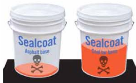
Figure 1: Relative amounts of PAHs in sealcoat products
