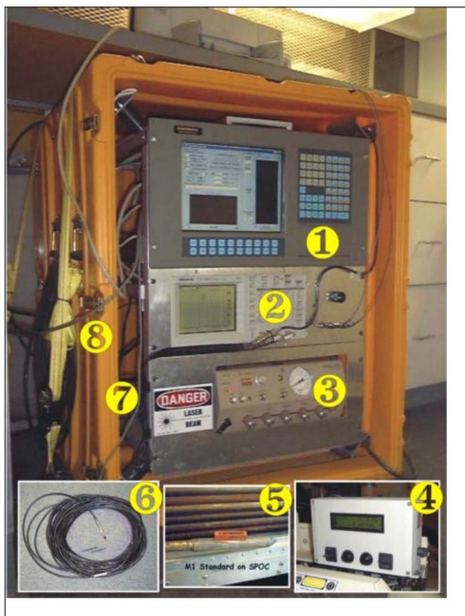
Figure 9. ROST system and key peripheral devices
