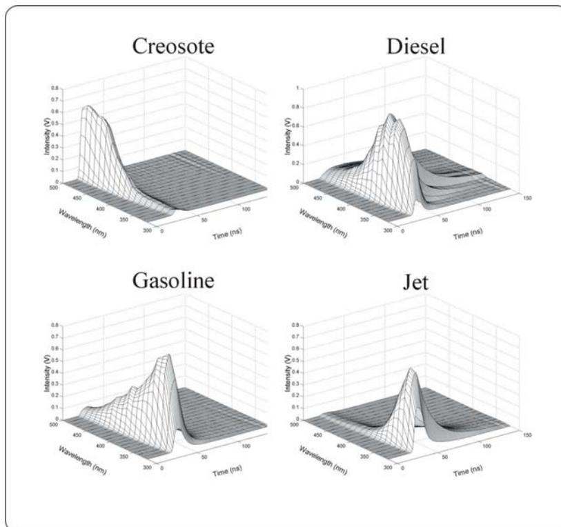
Figure 5. Example WTMs of common contaminants on sand
