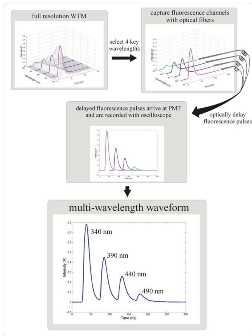
Figure 6. Multi-wavelength waveform concept
