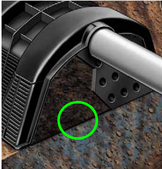
Gravel Drain Rock
