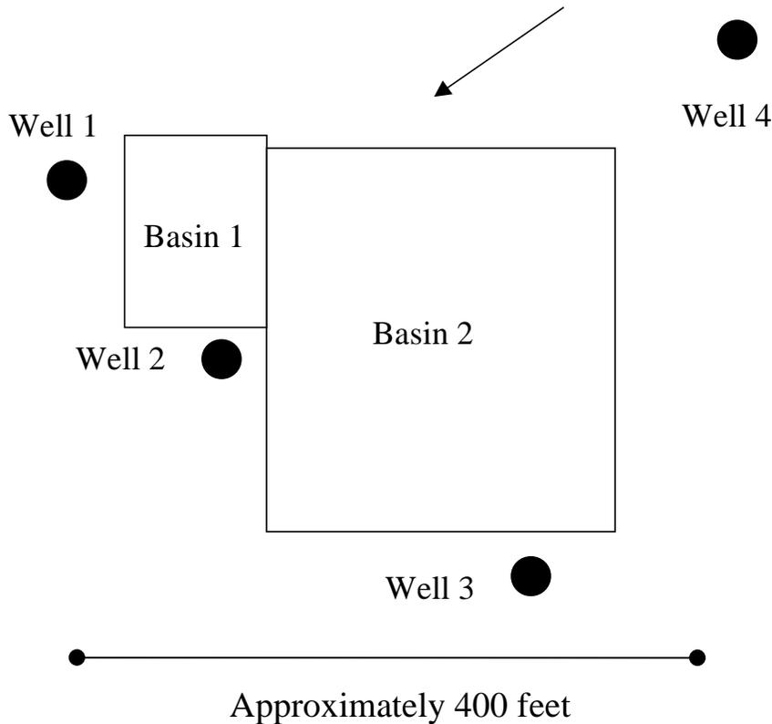
Figure 24: Location of monitoring wells, manure basins, and ground water flow direction (arrow) at site EM5.
