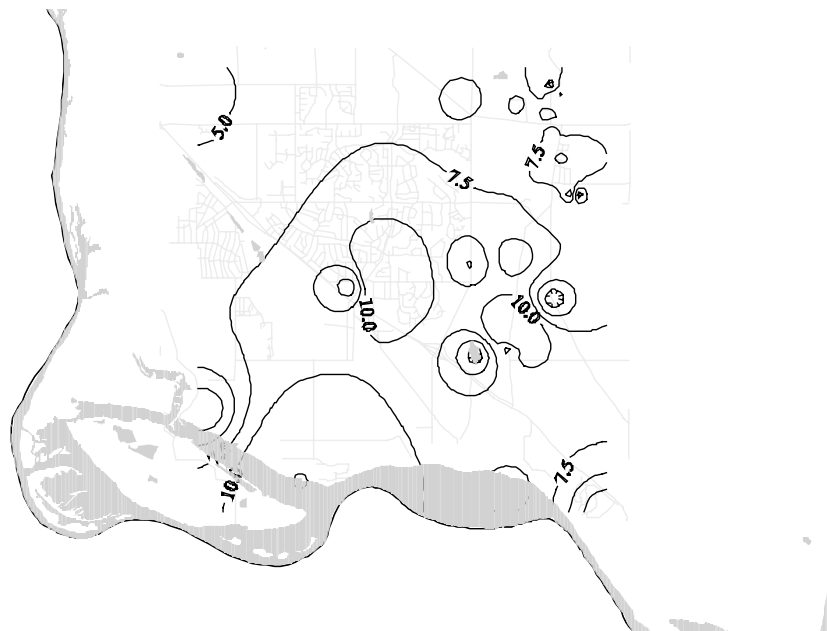
Figure 7: Distribution of nitrate in nitrate-vulnerable wells sampled for this study. All aquifers are considered together. Contours show concentrations in mg/l. A nitrate-vulnerable well is defined as having an Eh greater than 250 mV, a dissolved oxygen concentration greater than 1.0 mg/l, and an iron concentration less than 0.1 mg/l (MPCA, 1999a). Nitrate introduced to these wells will not be denitrified because of the presence of oxidizing conditions in the water.
