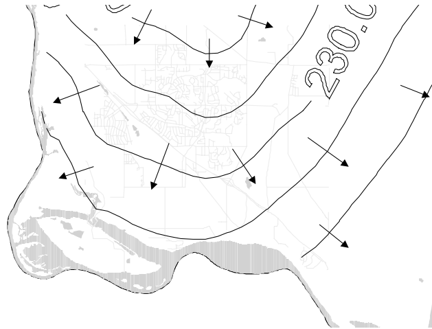
Figure 3: Ground water flow within the Prairie du Chien-Jordan aquifer. Contour intervals are 15 meters or 47.4 feet.
