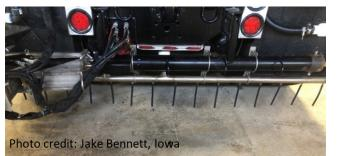
Figure 18: Stream nozzles for anti-icing
