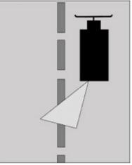
Figure 26: Sand spread pattern
