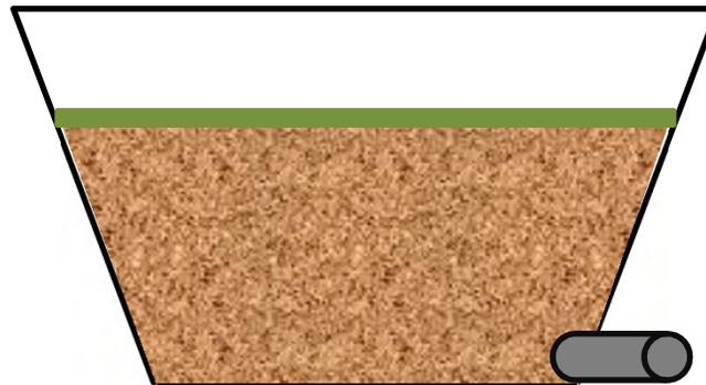
Bottom Drain Tile (Biofiltration)
