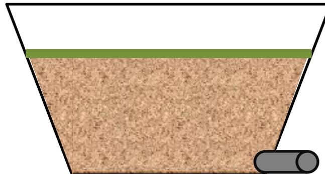
Bottom Drain Tile (Biofiltration)
