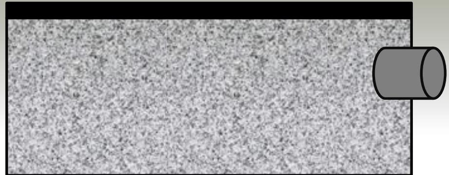
Typical (Elevated Drain Tile/Outlet)
