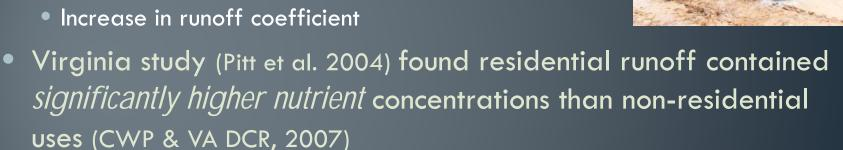
Disturbed and intensively managed pervious areas may result in elevated nutrient levels in stormwater
