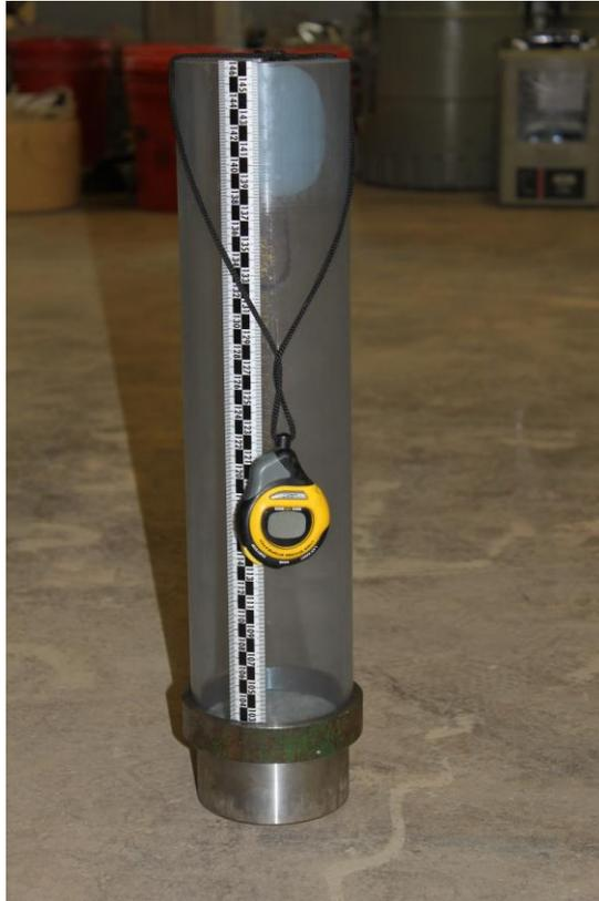
**Figure 1: Modified Philip-Dunne Infiltrometer**
