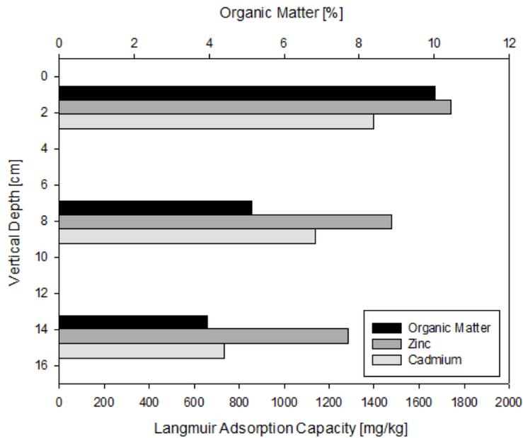
**Figure 14. Zinc and cadmium adsorption capacities (Langmuir) as a function of depth and organic matter content.**
