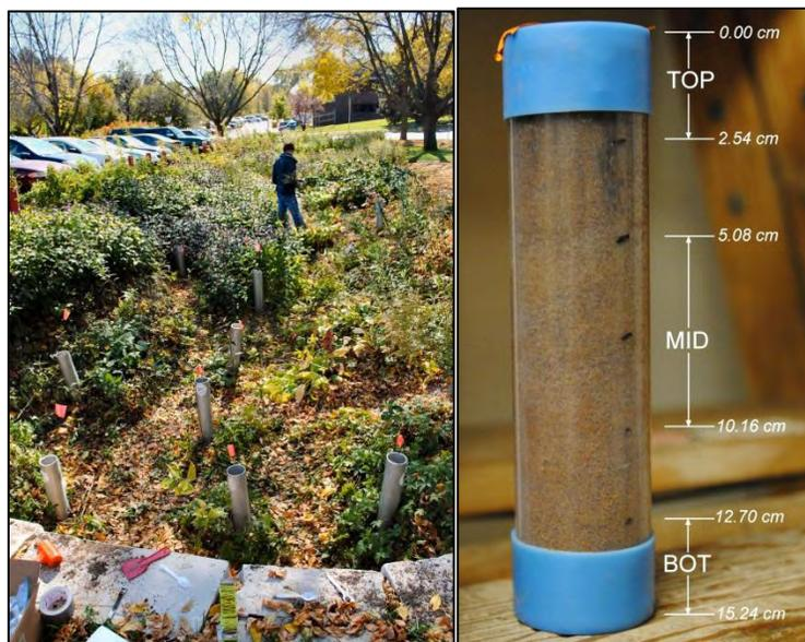
**Figure 2. Running infiltration tests on a bioretention practice to map its spatial capability to infiltrate water (Left Picture) and soil core collected to determine the depth of higher metals concentration (Right Picture)**
