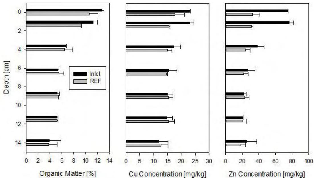
**Figure 13. Profiles of organic matter, copper, and zinc concentrations at two different cores in the St. Paul campus bioretention practice. Samples were collected near the inlet pipes (INLET) and from a reference location outside the bioretention practice (REF).**
