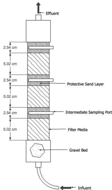
**Figure 1. Column Diagram**
