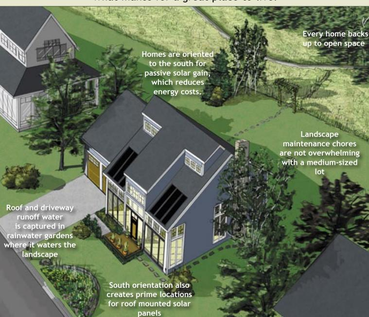
With increasing energy costs, it is even more important to take advantage of free heating - the sun! This passive solar home works to store the heat of the sun collected during the day in the floor of the south facing rooms. At night, this stored energy radiates to heat the home (for free). In order to harvest this free energy, it is important to orient homes to the south and streets east-to-west in a new development.
