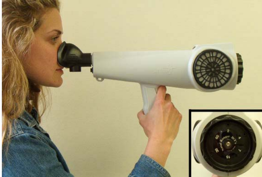
Figure 4.3. The Nasal Ranger® Field Olfactometer (St. Croix Sensory, Inc.). The inset picture shows a close-up of the orifice dial, which is located right side of the Nasal Ranger in this photo.
