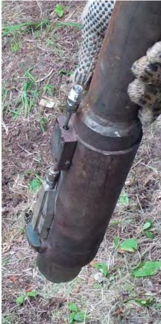
The Freeze Shoe seals the end of a core sample enabling a water sample to be obtained from precisely documented depth.
