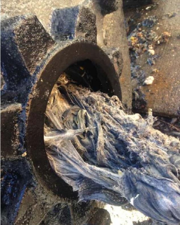
A wipes clog protruding from the intake side of a submersible wastewater pump in the Redwood Falls wastewater treatment plant.
