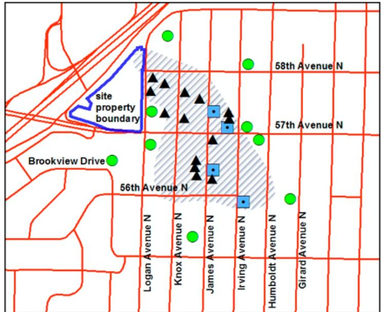
Figure 1: Location of Sub-Slab Vapor Sampling Locations
