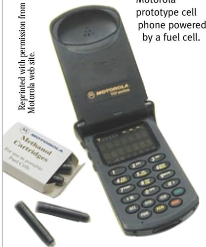
Motorola prototype cell phone powered by a fuel cell.
