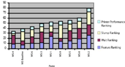
Summary graphs of the print test comparing how well each of the pastes printed onto the test card.
