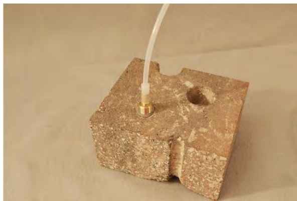
Figure 5. Vapor Pin™ sample connection.
