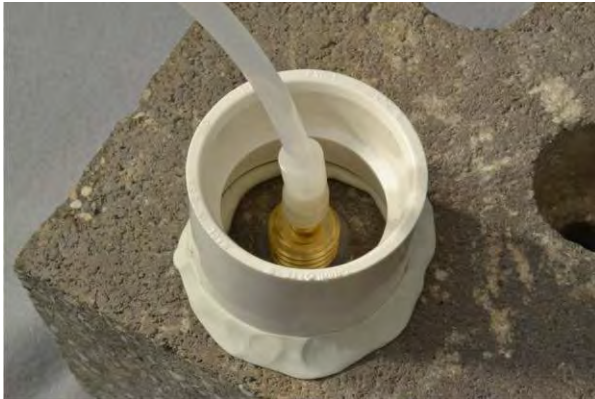
Figure 6. Water dam used for leak detection.
