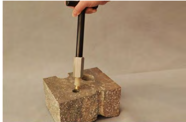
Figure 8. Extracted Vapor Pin™.
