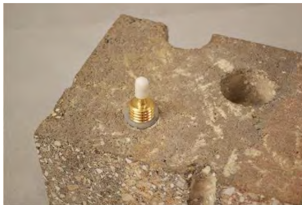
Figure 4. Installed Vapor Pin™.
