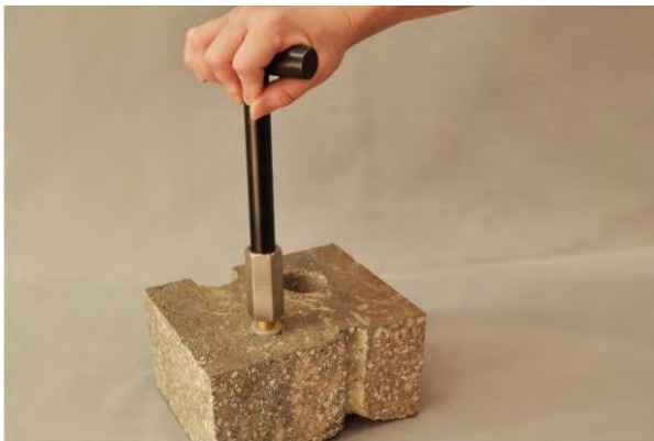
Figure 7. Removing the Vapor Pin™.
