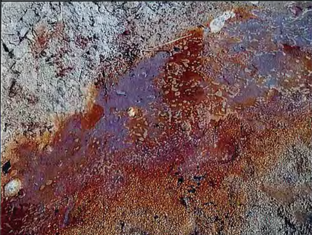
6a: SedOU: Iron bacteria sheen in water flowing near northeast corner Stryker Bay cap.
