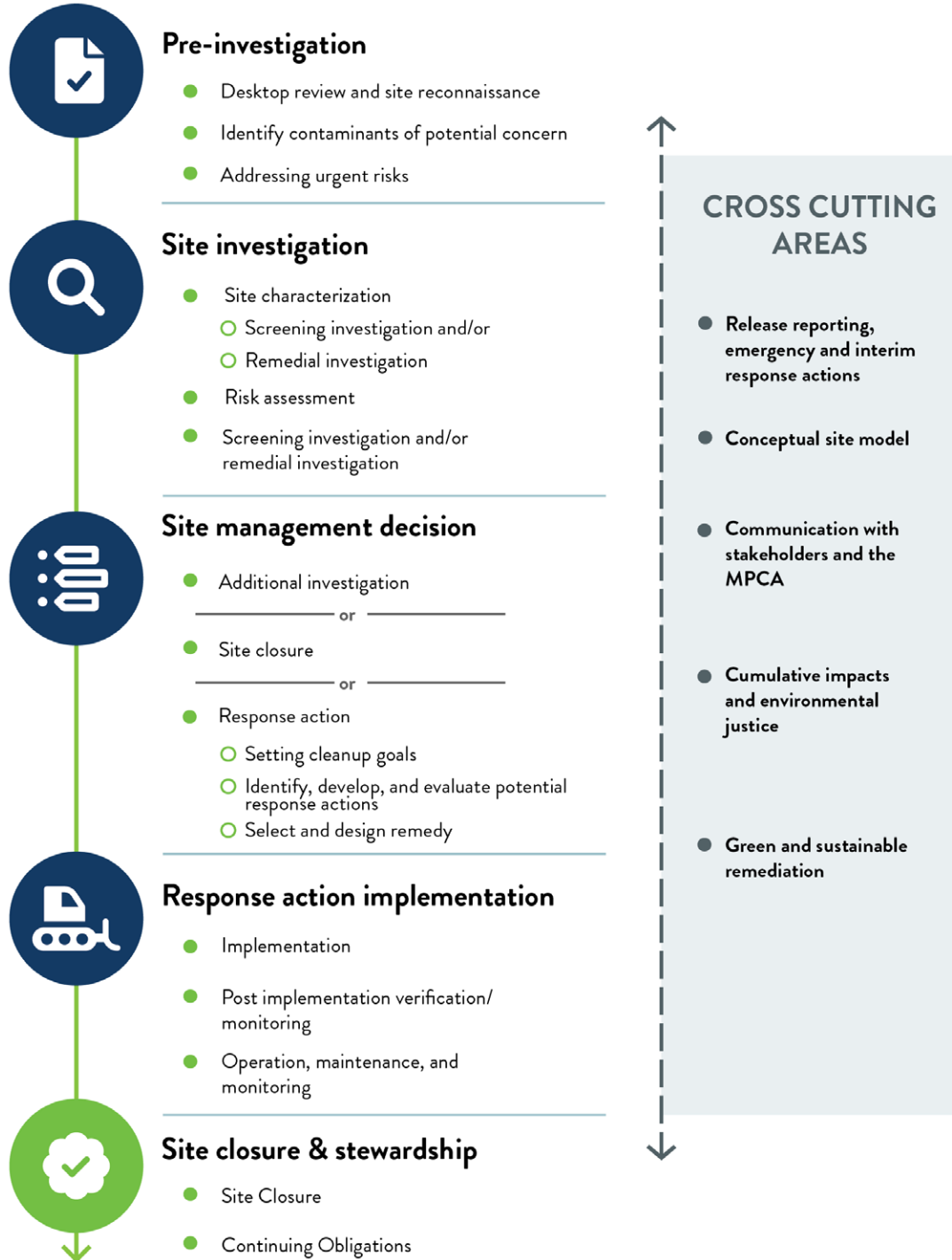
Figure 1 – Overview of the MERLA Remediation Process
