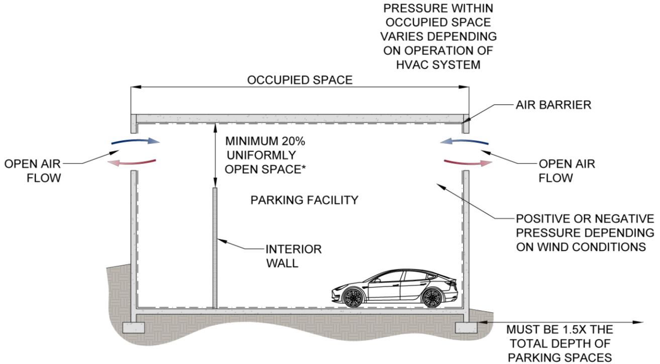
\*CODE REQUIRES OPEN SPACES TO BE AT LEAST 20% OF WALL AREA ON AT LEAST TWO SIDES. AGGREGATE OPEN AREA MUST BE 40% OF TOTAL PERIMETER.
