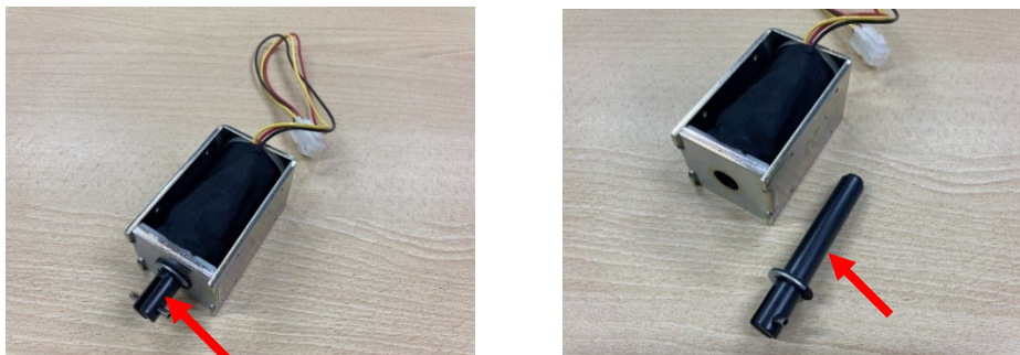
Figure 2.1.6. plunger of the solenoid motor and the bobbin pipe
