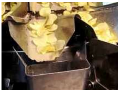
Example of oil accumulation (Food contact part is a flat stainless steel without coating)
