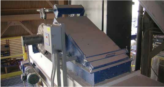
CPV-2 - Weigh belt feeder with limestone dust 800 cfm (1,359 m³/h)
