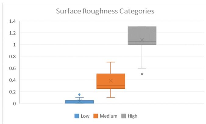
Figure 3. Box and whisker plot of the MSST surface roughness categories
