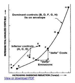
*Example:* Eight technically feasible control options for analysis are listed. These are represented as A through H in Figure 2. The dominant set of control options, B, D, F, G, and H, represent the least-cost envelope, as we depict by the cost curve connecting them. Points A, C and E are inferior options, and you should not use them in calculating incremental cost effectiveness. Points A, C and E represent inferior controls because B will buy more emissions reductions for less money than A;
