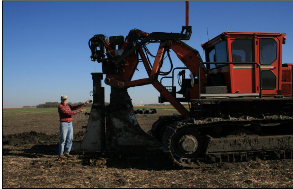
Equipment used to bury continuous plastic drain tile in fields.
