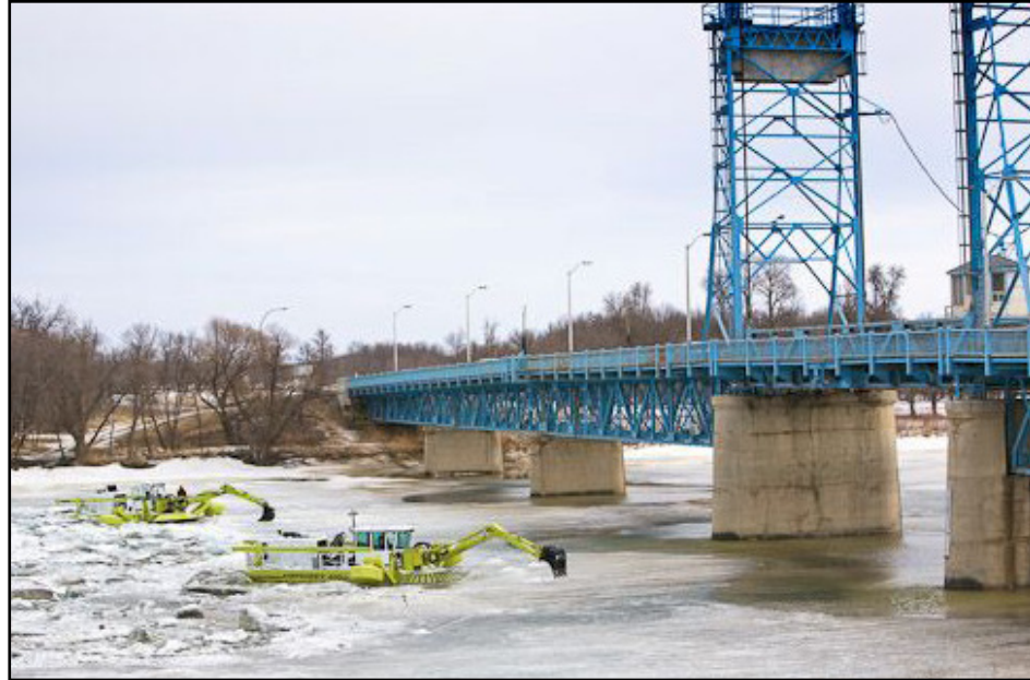
Amphibidex machines being used in Manitoba to break up ice on the Red River, 2009.
