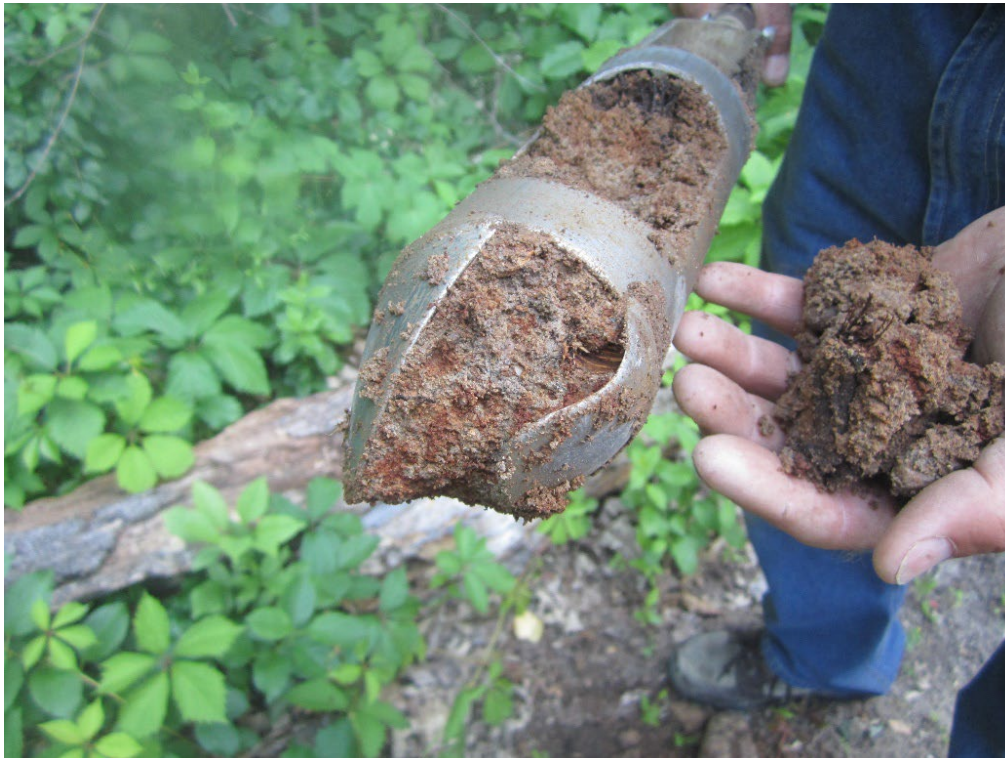
Figure 3. A hand auger tool is used during a soil observation
