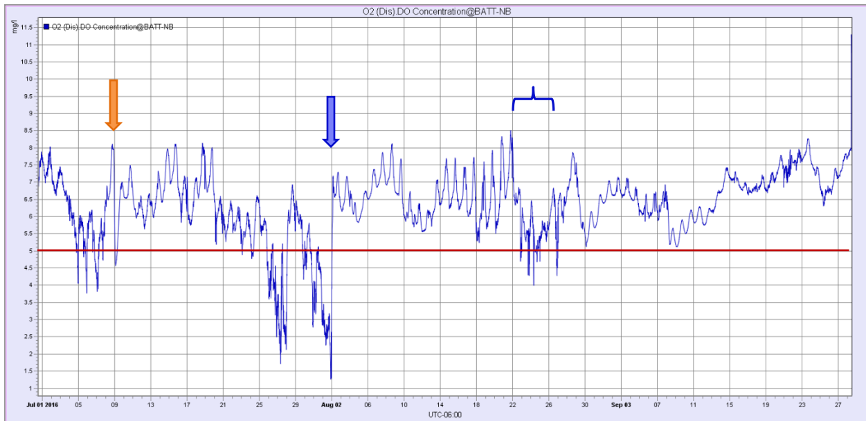
Figure 17. Continuously-recorded DO data at S003-962 from July 1 - Sept. 28, 2016 - collected by Red Lake DNR. The orange arrow points to abrupt change on 7/8 - 7/9, and the blue arrow points to abrupt change on 8/2. Compare with Figure 16. The red line is at the standard, 5.0 mg/L.
