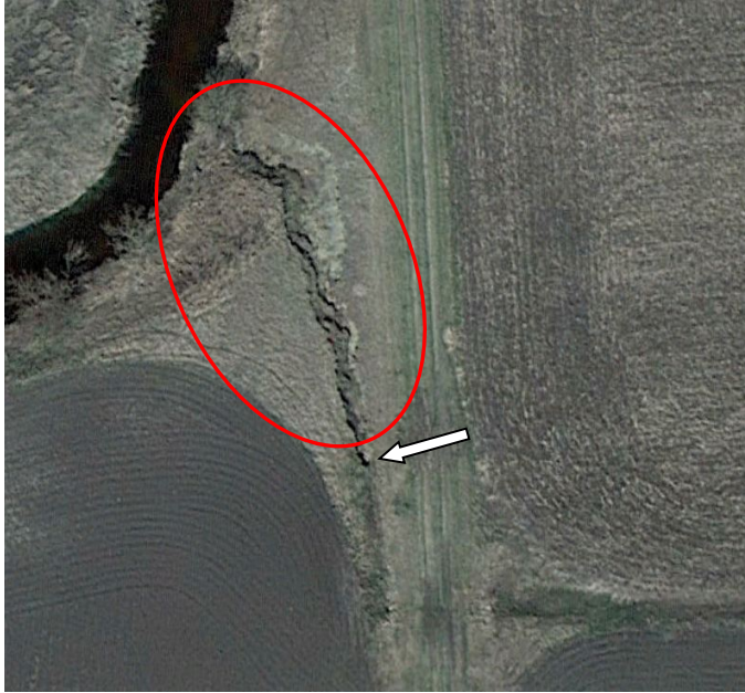
Figure 21. Field gully along the creek bank. The white arrow points to the nick point which is migrating away from the creek.
