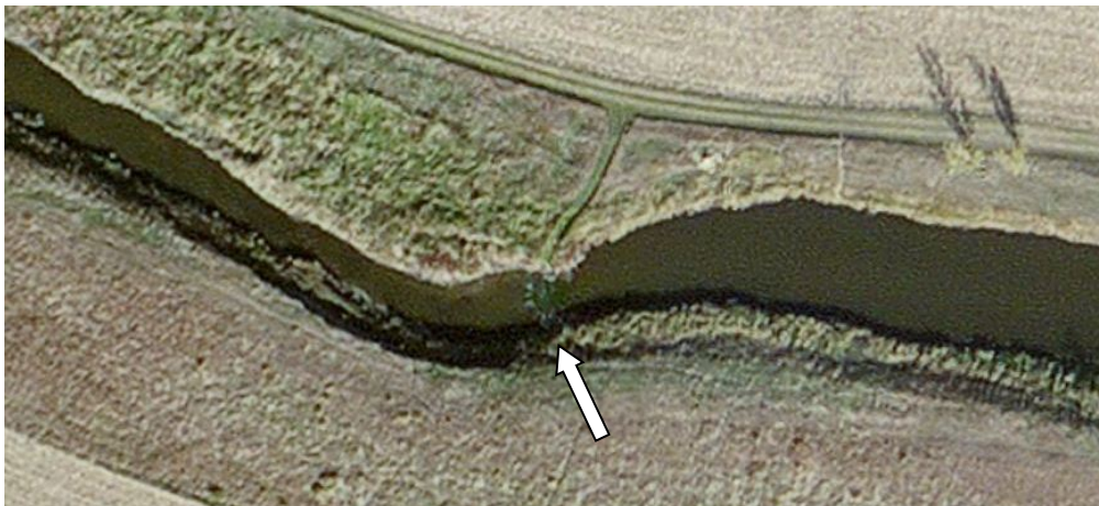
Figure 30. An apparently-created structure (trail leads to it), which may be a barrier to fish migration. Note the much wider channel on the upstream side, meaning the structure is ponding water. The convex shape of the structure is also diverting part of the flow into the south bank and causing erosion.
