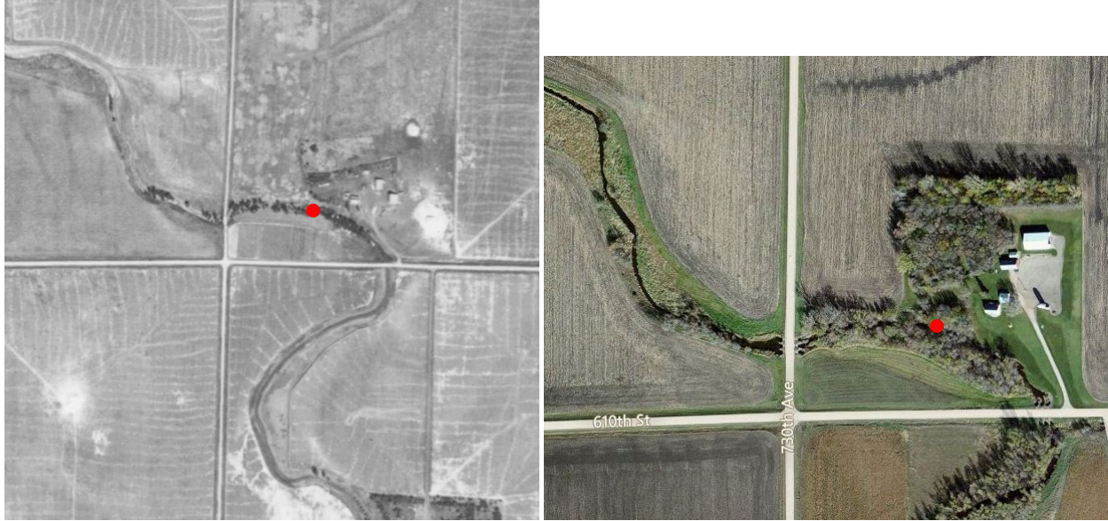
Figure 15. 1938 (L) and 2013 (R) aerial photos of 10RD057. The channel appears to have been smoothed all along this AUID. The forested patch that exists along the sampled reach presently was just beginning to grow up in 1938, likely the result of this early homestead adjacent to the young trees. The red dot denotes the center of the biological reach.
