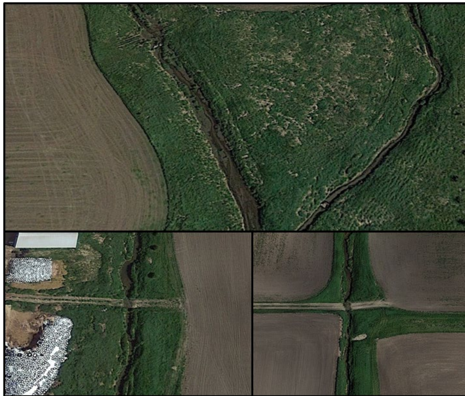
Figure 16: Private crossings near station 15CD012; it is unclear if these locations are affecting fish passage. Some of these crossings are located on AUID 507, while others are located on neighboring AUIDs. Notice the top photo has a crossing in the upper left corner and an unknown potential barrier in the lower right corner.
