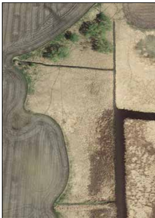
Figure 24. Small direct ditches (perhaps tile line outlets) inputting field runoff directly to the channel.
