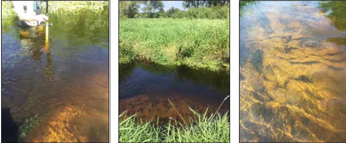
Figure 70. Pool Study XS resurvey, August 22, 2018. Sandy deposition and point bar development.
