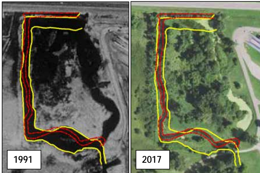
Figure 83. Yellow dots pinpoint the longitudinal profile and cross sectional survey data collected. Image courtesy of Google Earth, 2015.
