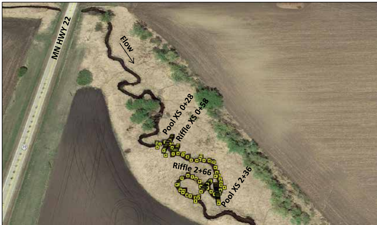
Figure 67. Location of Battle Creek geomorphic survey site; 2018 image courtesy of Google Earth. 2+66 is the classification riffle.
