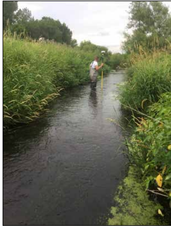
Figure 87. Along the upper reach survey, collecting a bankfull survey elevation point (left) and lower reach survey in right-of-way with narrower channel (right).
