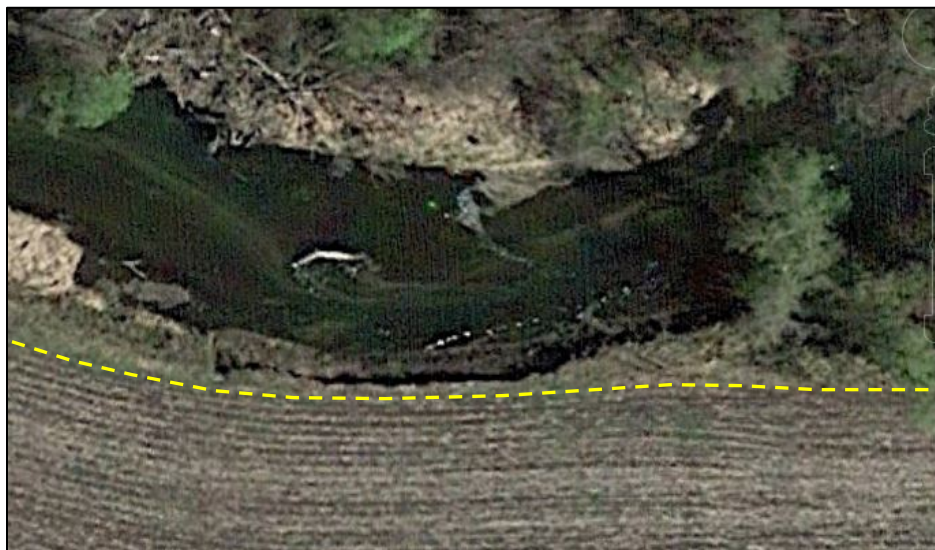
Figure 7. Example of bank erosion along a field edge with almost no buffer (Photo is spring 2015). Such erosion is a source of excess sediment. This erosion is upstream a ways from location shown in Figure 6. The dashed yellow line is the edge of active cultivation.
