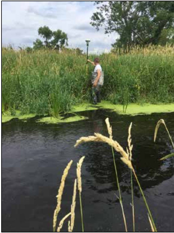
Figure 87. Along the upper reach survey, collecting a bankfull survey elevation point (left) and lower reach survey in right-of-way with narrower channel (right).
