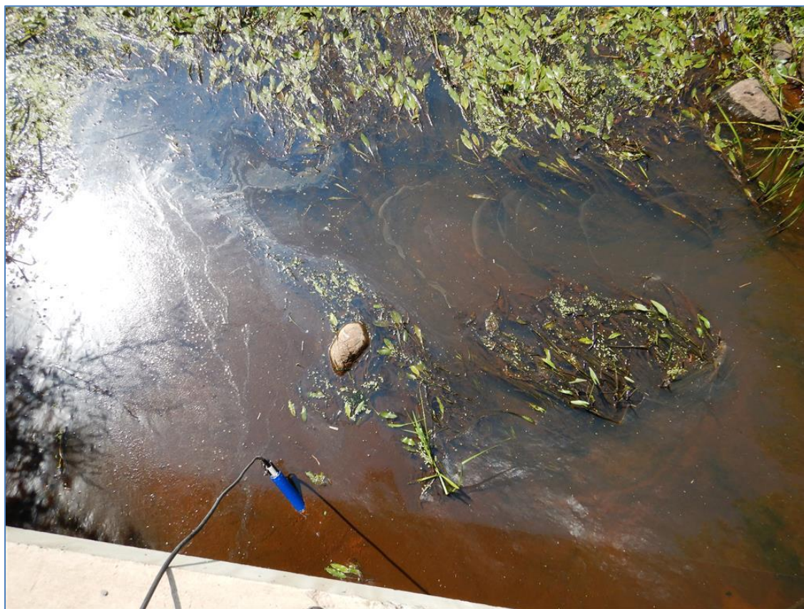
Figure 11. Evidence of iron in Big Mink Creek at 16UM107 on 8/16/2018. Ferric iron precipitate is causing the orange coloration of the water and an oily sheen on the surface. Dissolved oxygen was 0.36mg/L and specific conductance was 551 \mu S/cm.
