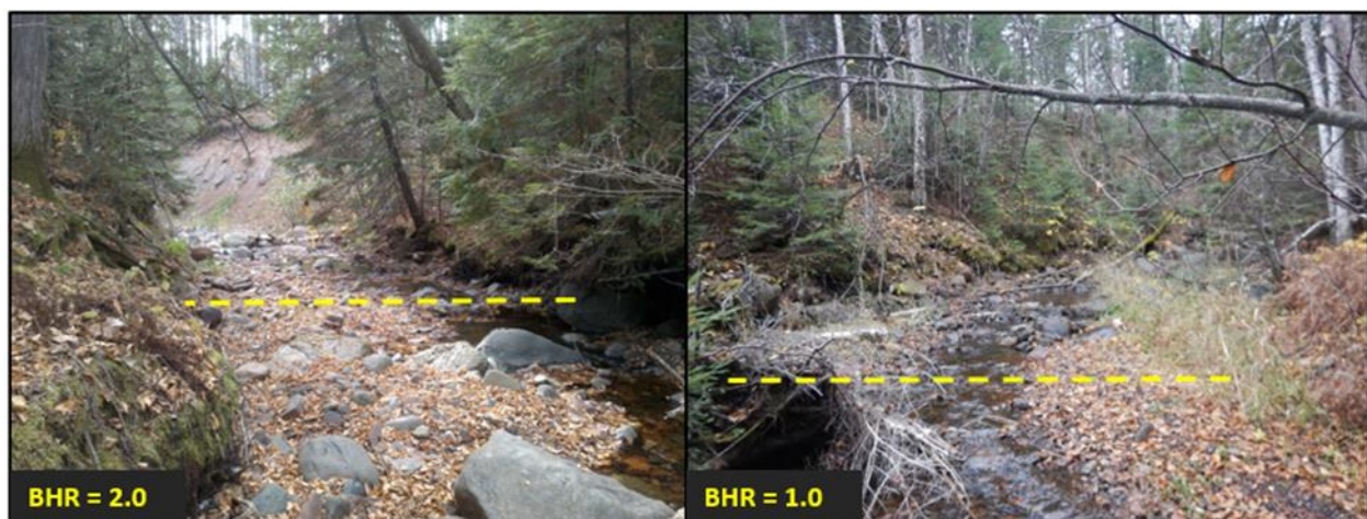
Figure 52. Examples of BHR values of 2.0, deeply incised (left), and 1.0, stable and connected to floodplain (right), in Woods Creek. Yellow line approximates bankfull height. Predicted erosion rates were higher in reaches with high BHR values.
