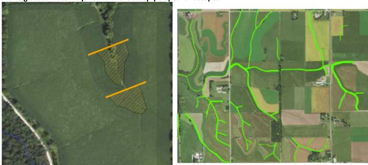
Figure 41. Example outputs from RRW ACPF and SPI tool. Left shows two potential WASCOB locations. Right shows grassed waterways found in the steeply sloped landscapes.
