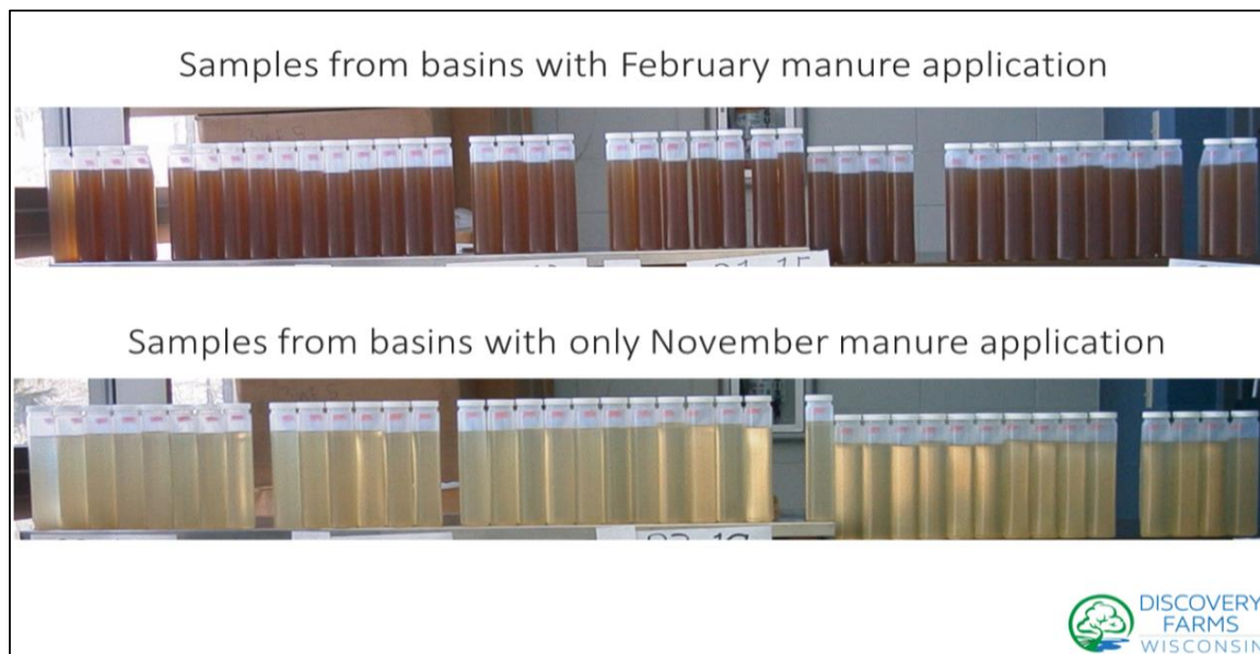
Figure 23. Comparison of runoff when manure is applied in early winter and late winter (photo from Discovery Farms).
