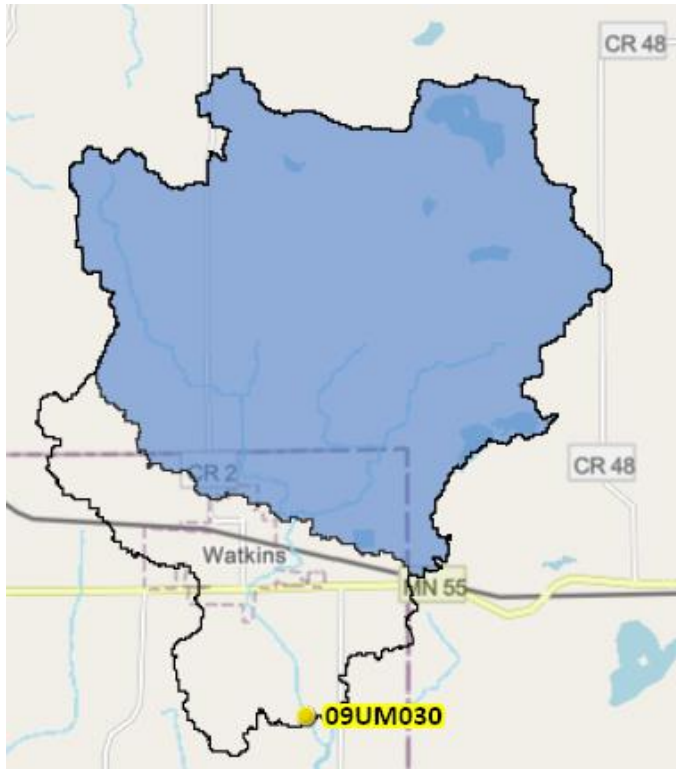
Figure 32. County Ditch 20 current drainage area, with additional drainage area from channelization denoted in blue. Credit: USGS Stream Stats.
