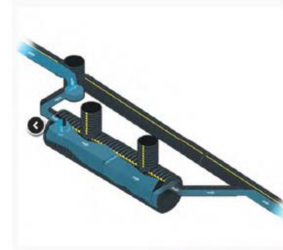
Off-Line Stormwater Quality Tank Concept (Prinsco)
