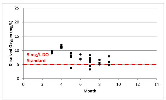
Figure 3-8. Seasonal variation of dissolved oxygen samples in Buffalo Creek measured before 9:00 a.m. The red dashed line indicates the 5 mg/L DO standard.
