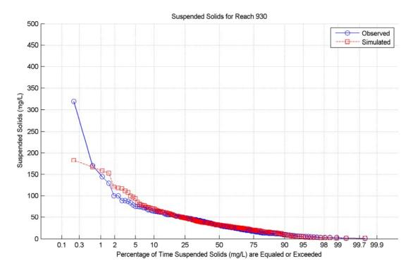
Figure B-1. Suspended Solids Concentration Duration Curve at Reach 930.
