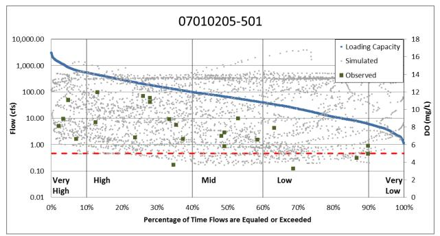
Figure 3-11. Dissolved oxygen samples taken before 9:00 a.m. in Buffalo Creek plotted on flow duration curve. The red dashed line indicates the 5 mg/L DO standard. Simulated DO values represent the daily minimum dissolved oxygen values.
