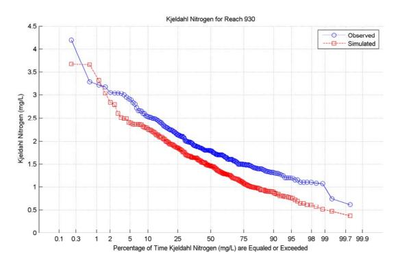
Figure B-28. Kjeldahl Nitrogen Concentration Duration Curve at Reach 930.
