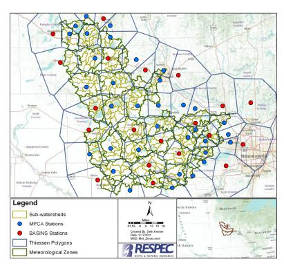
**Figure 2.** Aggregation of Subwatersheds Into Meteorological Zones Using the Thiessen Polygon Approach.
