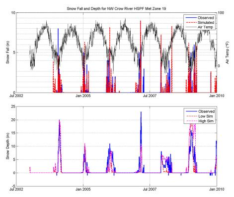
Figure 3. Snow Level (Top) and Snow Depth (Bottom) Calibration Figures.
