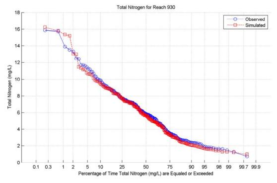
Figure B-19. Total Nitrogen Concentration Duration Curve at Reach 930.
