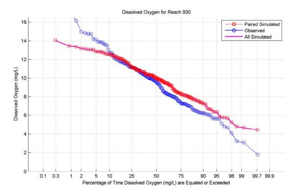
Figure B-7. Dissolved Oxygen Concentration Duration Curve at Reach 930.
