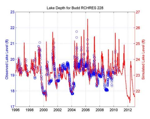
Figure 9. Lake-Level Calibration Example.
