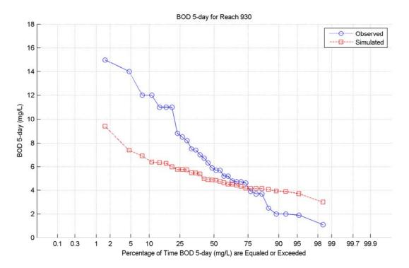
Figure B-10. BOD-5 Concentration Duration Curve at Reach 930.
