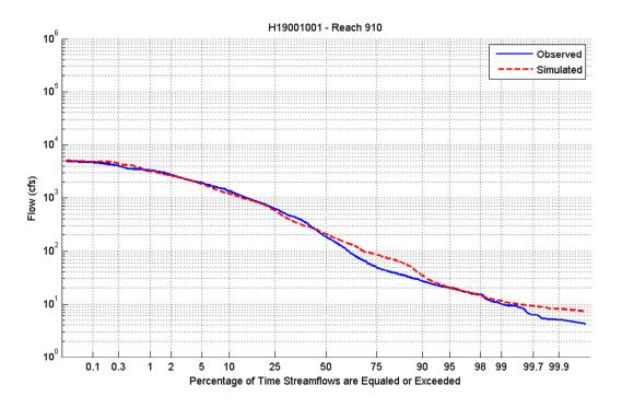
Figure B-11. Flow Duration Plot for Reach 910.
