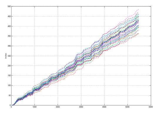
Figure 4. Mass Curve of Accumulated Precipitation Over Modeling Period in Days.
