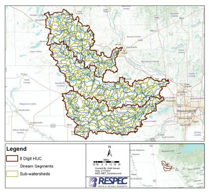
Figure 1. Subwatershed Stream Segmentation Refined From Level 7 Minor Watersheds.
