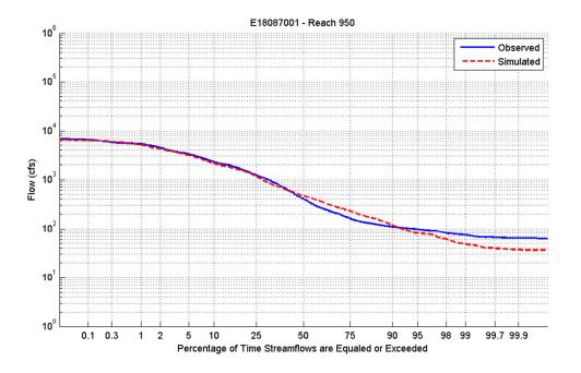
Figure B-15. Flow Duration Plot for Reach 950.
