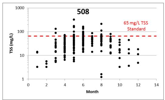
Figure 3-6. Seasonal variation of TSS at South Fork Crow River 07010205-508. The red dashed line indicates the South River Nutrient Region 65 mg/L TSS standard.4.3 Total Suspended Solids TMDLs
