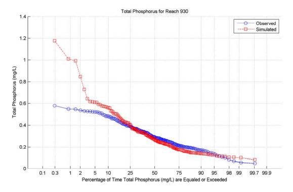
Figure B-13. Total Phosphorus Concentration Duration Curve at Reach 930.
