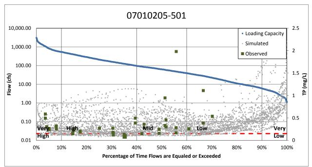
Figure 3-14. TP samples in Buffalo Creek plotted on flow duration curve. The red dashed line indicates the .015 mg/L proposed TP standard. Simulated TP values represent the daily average values.
