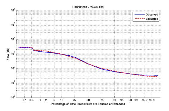
Figure B-3. Flow Duration Plot for Reach 430.
