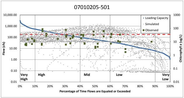
Figure 3-15. Chlorophyll-a samples in Buffalo Creek plotted on flow duration curve. The red line indicates the 35 mg/L chlorophyll a standard. Simulated chlorophyll a values represent the daily average values.
