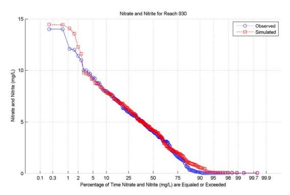
Figure B-22. Nitrate and Nitrite Concentration Duration Curve at Reach 930.
