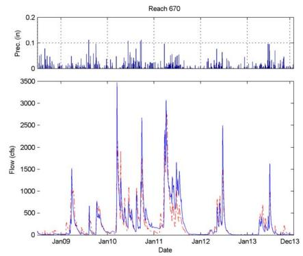
Figure A-6. Discharge Time Series at Reach 670.
