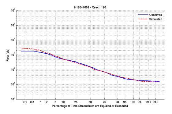
Figure A-3. Flow Duration Plot for Reach 190.
