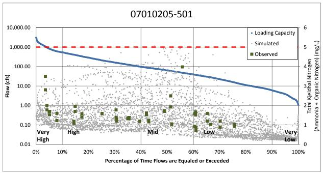
Figure 3-13. TKN samples in Buffalo Creek plotted on flow duration curve. Simulated TKN values represent the daily average values.
