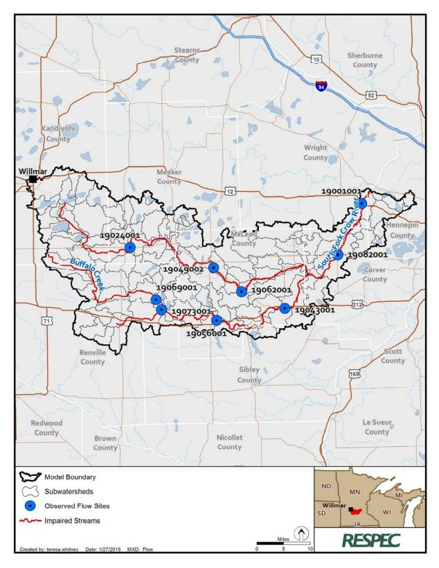
Figure 6. Flow Calibration Gages Within the South Fork Crow River Watershed.
