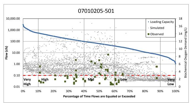
Figure 3-12. BOD5 samples in Buffalo Creek plotted on flow duration curve. The red dashed line indicates the 3 mg/L proposed BOD5 standard. Simulated BOD5 represent the daily average values.
