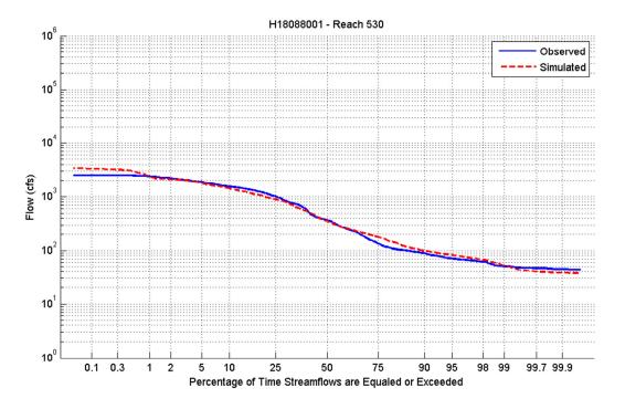
Figure B-7. Flow Duration Plot for Reach 530.
