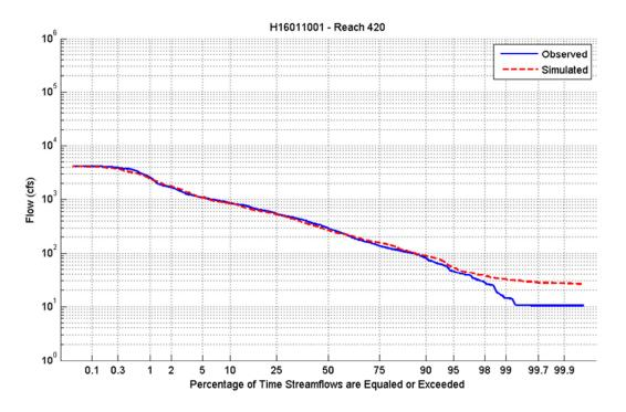
Figure A-15. Flow Duration Plot for Reach 420.
