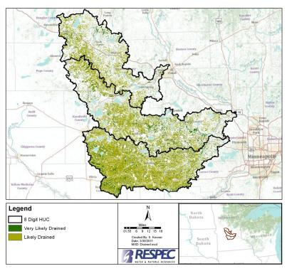
Figure 8. Cultivated Cropland Areas Most Likely to Be Drained With Artificial Drainage.
