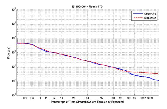
Figure A-19. Flow Duration Plot for Reach 470.
