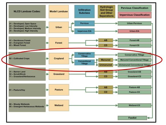
Figure 2. New Classification for the Crow and Sauk Watershed Model Applications.
