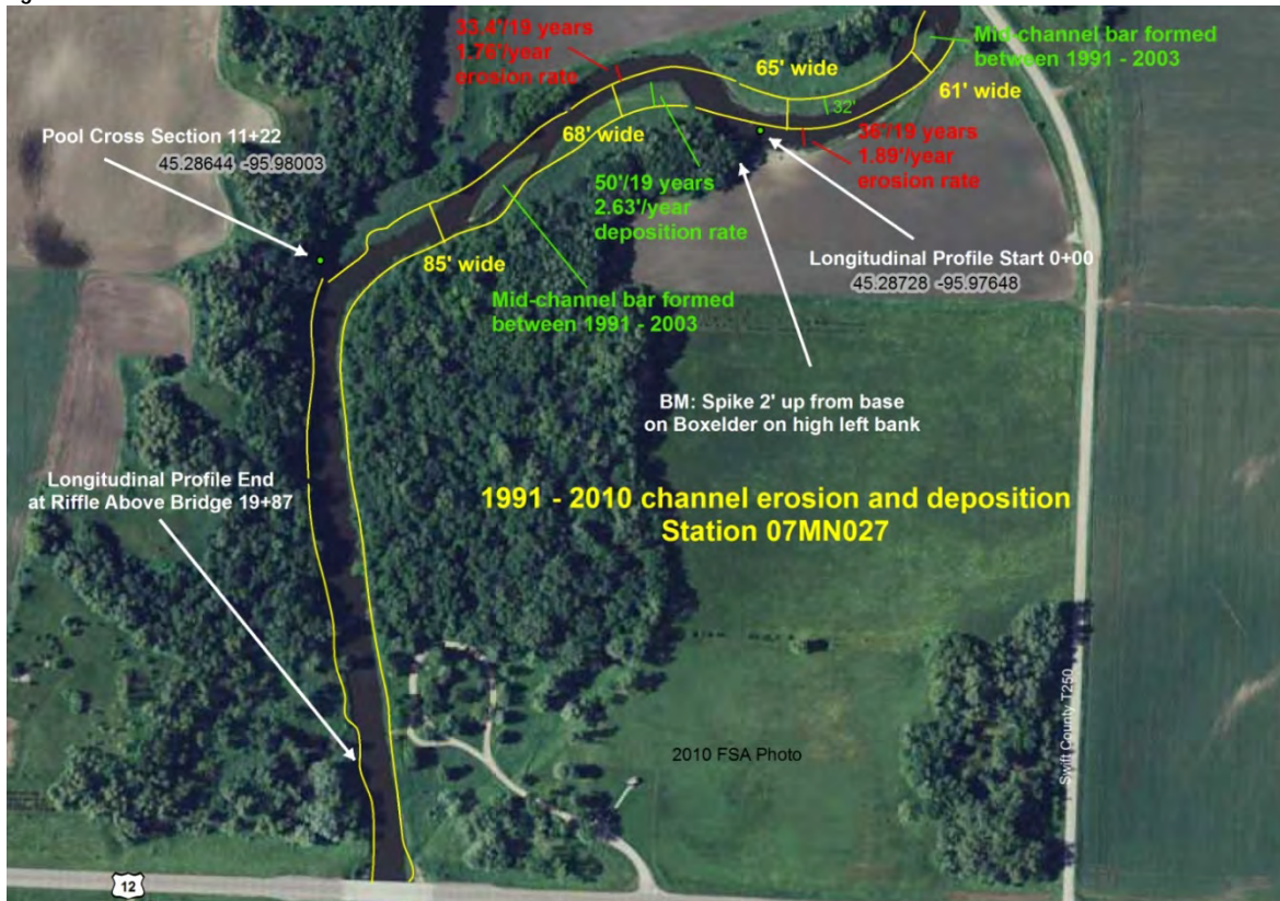
Figure 112. 2010 aerial photograph with 1991 overlay at station 07MN027
