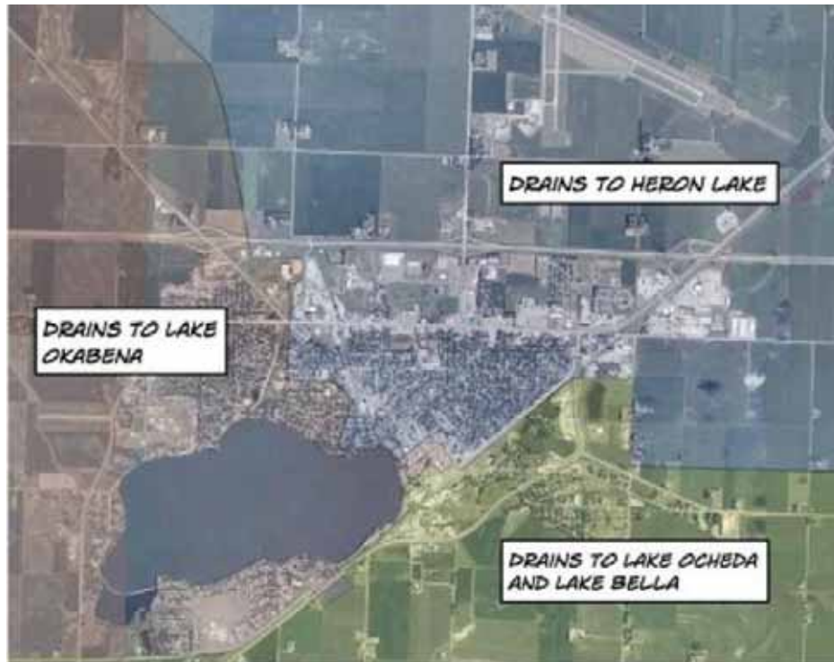
Figure 1: Worthington's Stormwater Drainage Map
