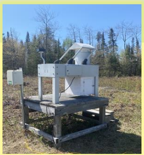
Hg Isotope Collectors Set-up for Lake Superior Assessment
