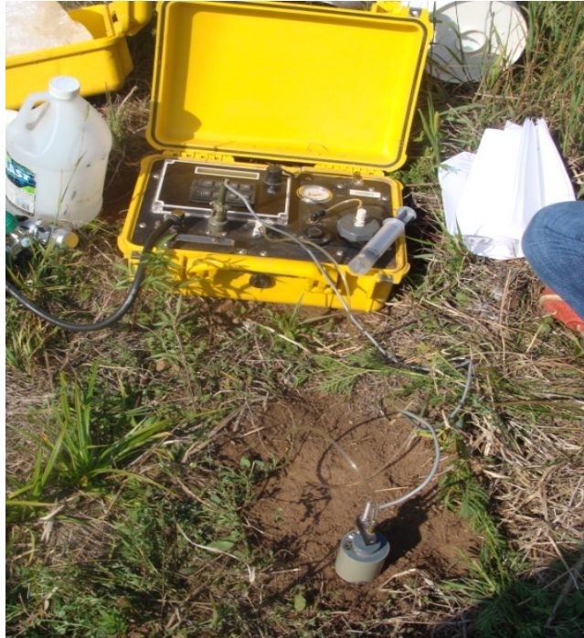
Figure 4. Cohesive strength meter measuring critical shear on a ski slope.
