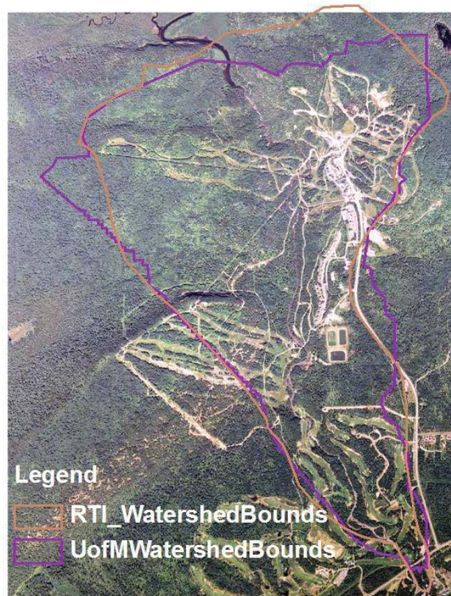
Figure 9. Watershed delineations for the Lower Poplar River watershed. One delineation is for the current effort (UofM) while the other one is for the RTI study (RTI, 2008).
