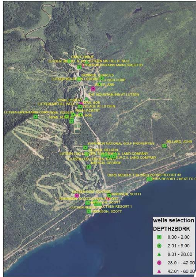
Figure 4. Map showing the depth to bedrock as indicated from the well logs for the locations shown.
