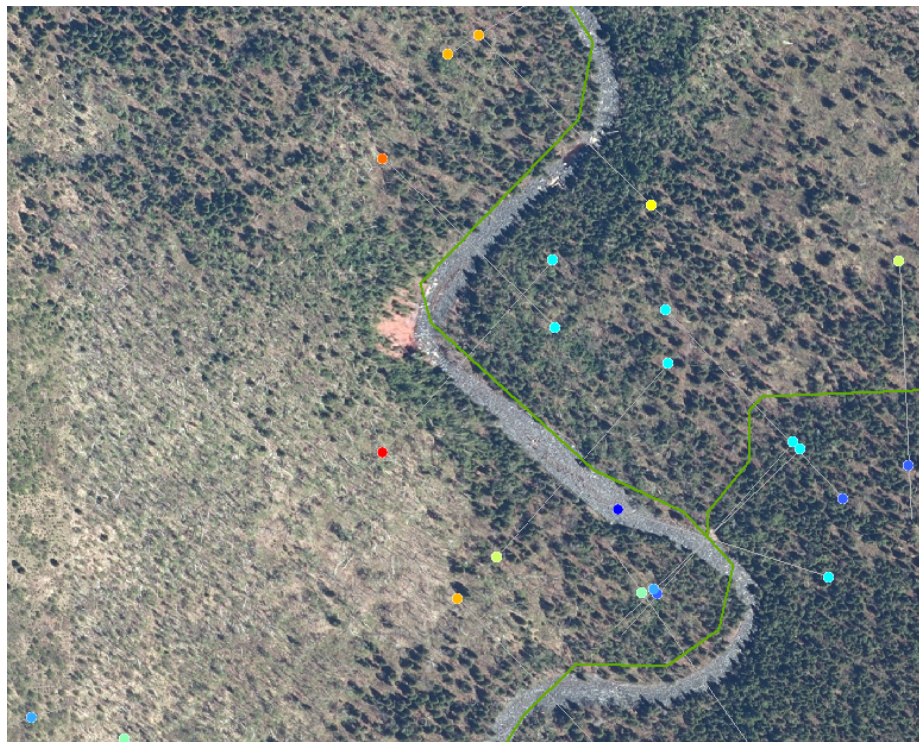
Figure 7: Slump in area indicated as high risk by stream context point methodology.
