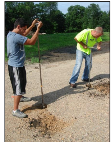
Above: A graduate student from the UMN and SET staff use augers to make holes for the lysimeters.
