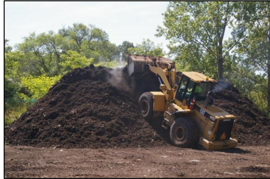
Above (left): SET staff tears down a pile from the active composting area of the site after it met PFRP. Above (right): SET staff creates a new pile in curing area of the site with the material that has met PFRP in the actively composting area of the site.
