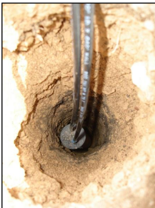
Above (left): View of a lysimeter in a 3' deep hole. Above (middle): A UMN graduate student pours the sealant into the lysimeter hole. Above (right): SET staff place lysimeter tubes in PVC pipe for added protection.
