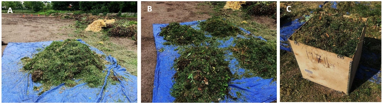
Figure 3. Grass/garden waste sampling process. A) Gross sample of grass/garden waste before mixing. B) Four subsamples. C) Tamped and leveled sample in weigh box.
