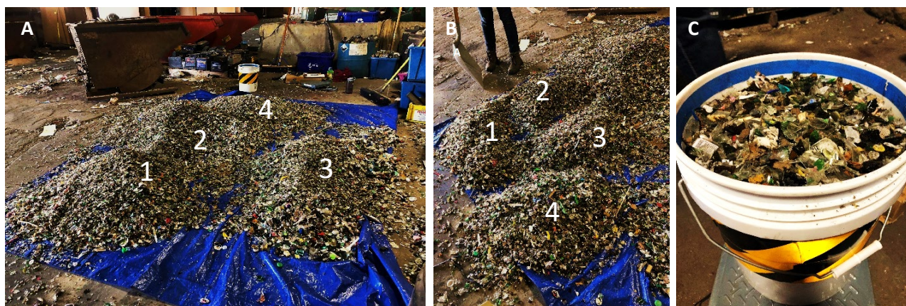
Figure 18. Glass sampling process. A) Four gross samples of glass on the work surface. B) Four subsamples from one gross sample. C) Tamped sample in 5-gallon bucket.
