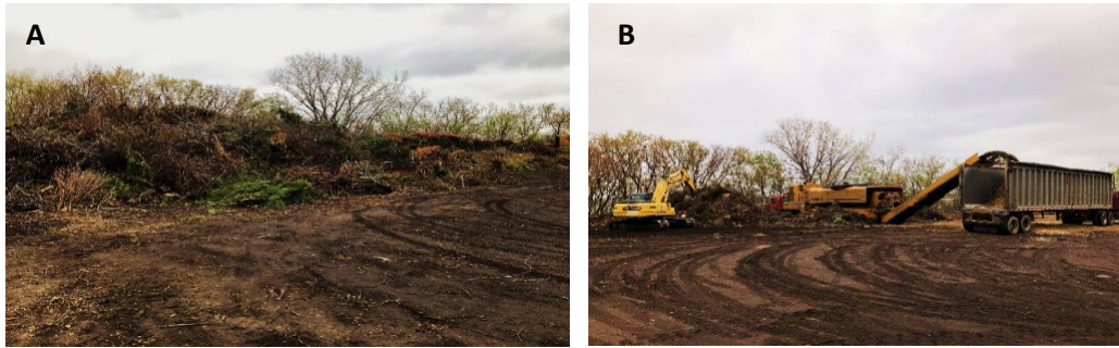
Figure 6. Brush sampling process. A) Large pile of loose brush before grinding. B) Brush chipping operation and filling trucks with chipped brush material.
