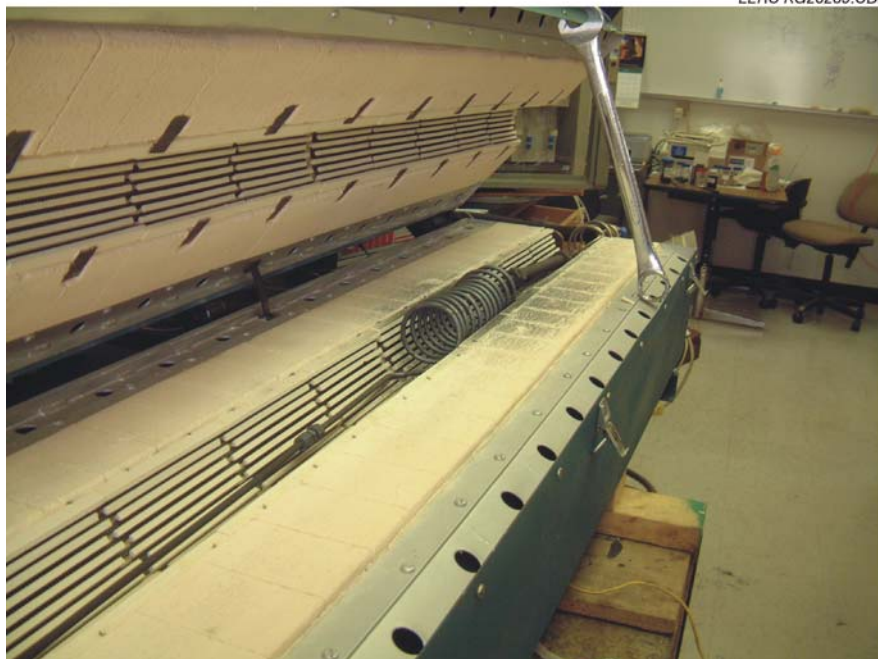
Figure 3. Photograph of the stainless steel heating coil and sample chamber in an oven.
