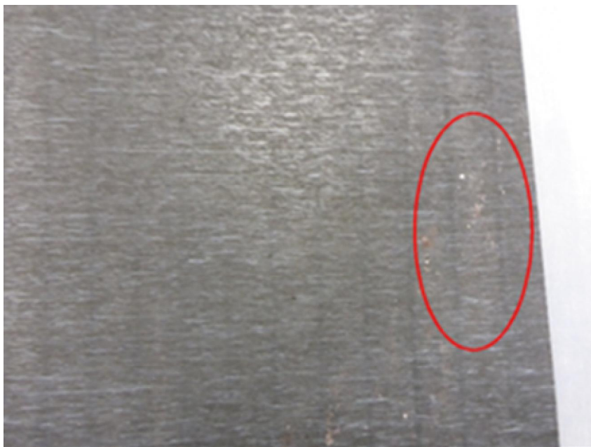
FIGURE 7: Magnified view of the circled image in Figure 6 - Sample of the visible particulate found on the SPC surface.
