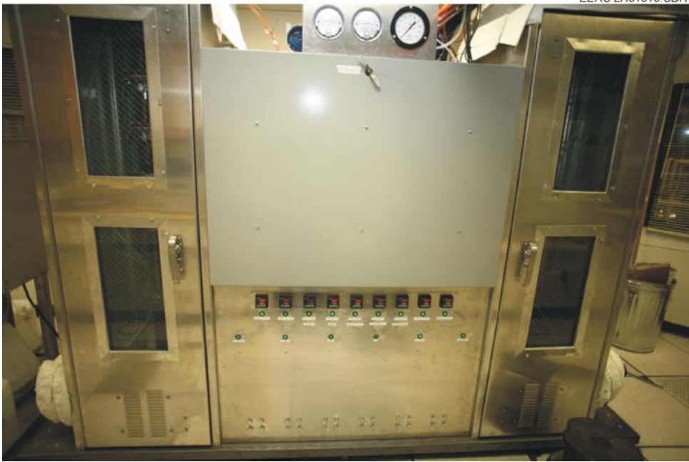
Figure 3. Photo of the column cabinets and the hot box.
