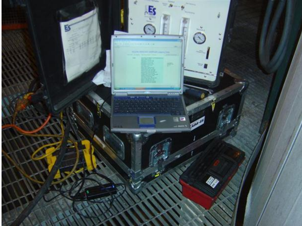
Figure 2: STM Sampling Console Setup at a Stack Sampling Location
