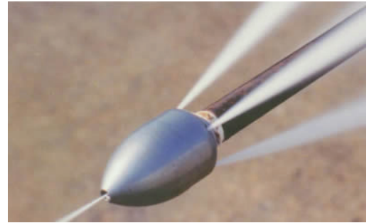
Figure 2-3: High velocity jet cleaner
